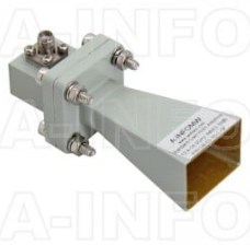
LB-62-10-C-3.5F Standard Gain Horn Antenna 12.4-18GHz 10dB Gain 3.5mm Female
